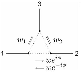
Y junction with built-in asymmetry between wires 1 and 2 let  $w_1 \neq w_2$
