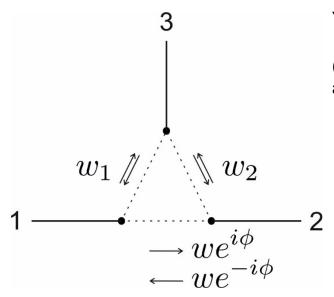
Y junction pierced by a magnetic flux  $\phi$
