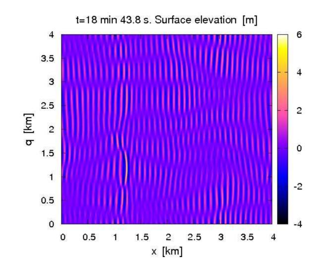
Figure 6: Experiment B2: the rogue wave is at  $x \approx 1.2$  km,  $q \approx [1.0 \cdots 1.3]$  km.
