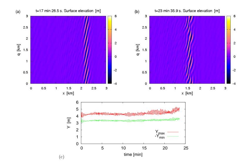
Figure 2: (a)-(b): Evolution of a perturbed high-amplitude oblique soliton into a zigzag structure; (c) Maximum and minimum elevation of the oblique soliton vs. time.
