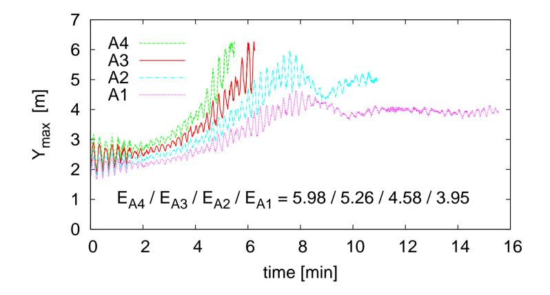
Figure 3: Maximum elevation of the free surface vs. time in the numerical experiments A1-A4.
