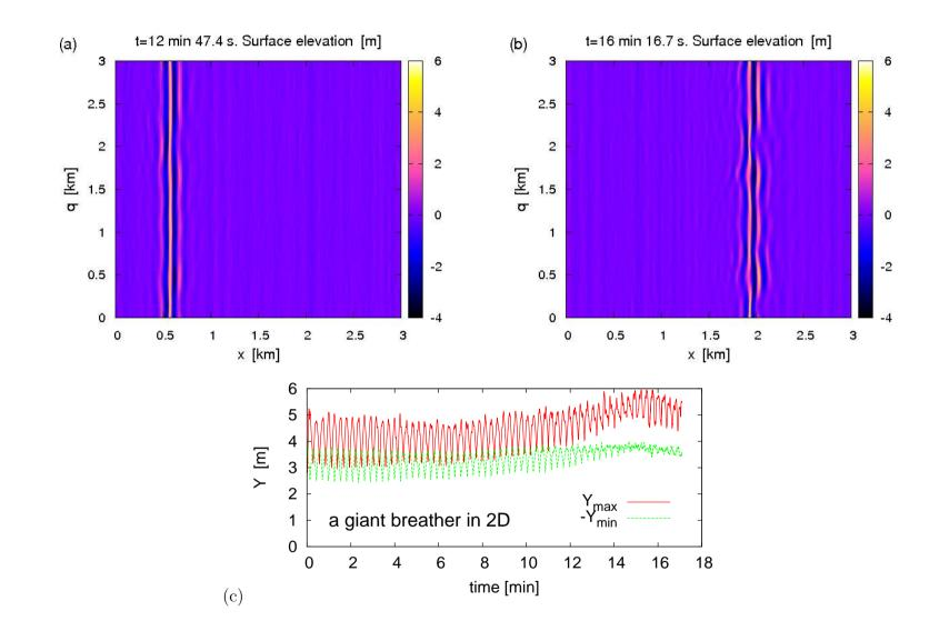
Figure 1: (a)-(b): Evolution of a perturbed giant breather in 2D; (c) Maximum and minimum elevation of the giant breather vs. time.
