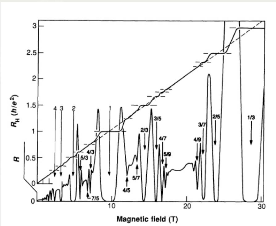
Hall( $R_H$ ) and longitudinal ( $R$ ) resistances as functions of the applied perpendicular magnetic field  $B$  at fixed temperature and electron concentration.
