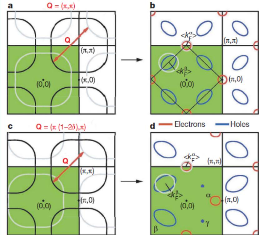
Figure 4 | Fermi surface reconstruction in  $\text{YBa}_2\text{Cu}_3\text{O}_{6.51}$ . a, Schematic Fermi surface reconstruction for a commensurate ordering wavevector  $\mathbf{Q} = (\pi, \pi)$  and nominal doping  $p_{\text{nom}} = 0.1$  in the extended Brillouin zone
