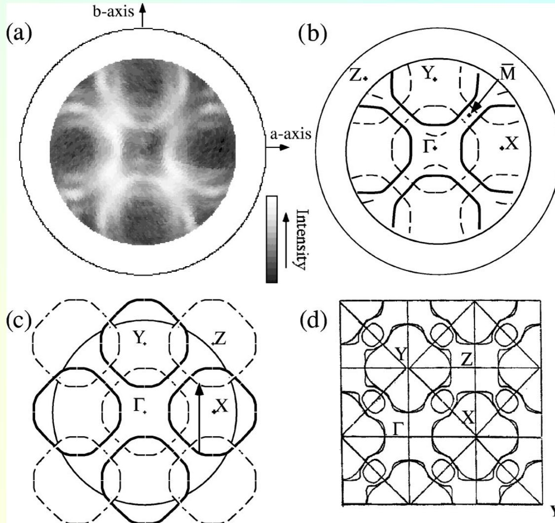
The Fermi surface of near optimally doped  $\text{Bi}_2\text{Sr}_2\text{CaCu}_2\text{O}_{8+\delta}$  (a) integrated intensity map (10-meV window centered at  $E_F$ ) for Bi2212 at 300 K obtained with 21.2-eV photons (HeI line); (b),(c) superposition of the main Fermi surface (thick lines) and of its  $(p,p)$  translation (thin dashed lines) due to backfolded shadow bands; (d) Fermi surface calculated by Massidda *et al.* (1988).
